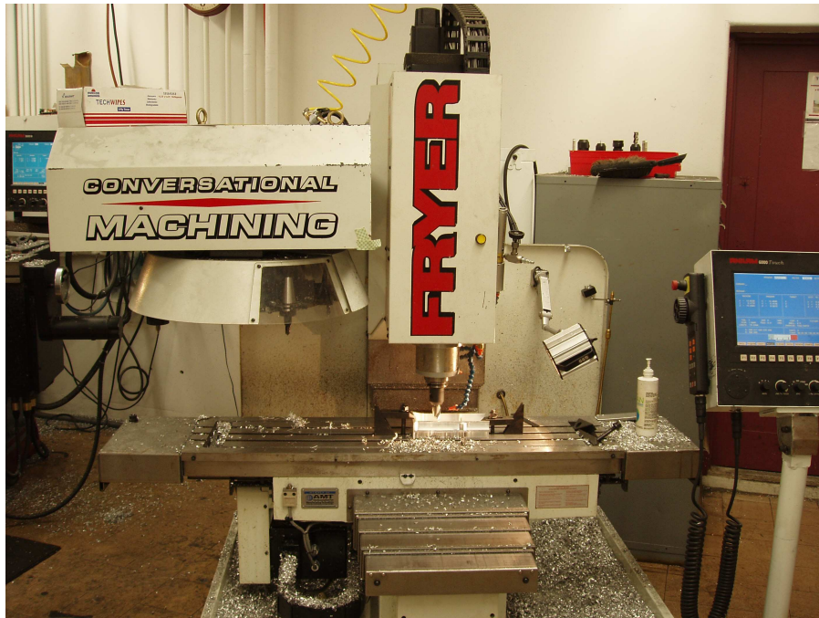
Figure 2.13 F-15: milling using Fryer MB-10
